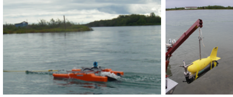
Figure 2: Dopppcat platform for down looking Nortek Aquadopp velocity profiler (left) and sounding weight platform for Nortek Vector velocimeter (right) at Igiugig, AK.
